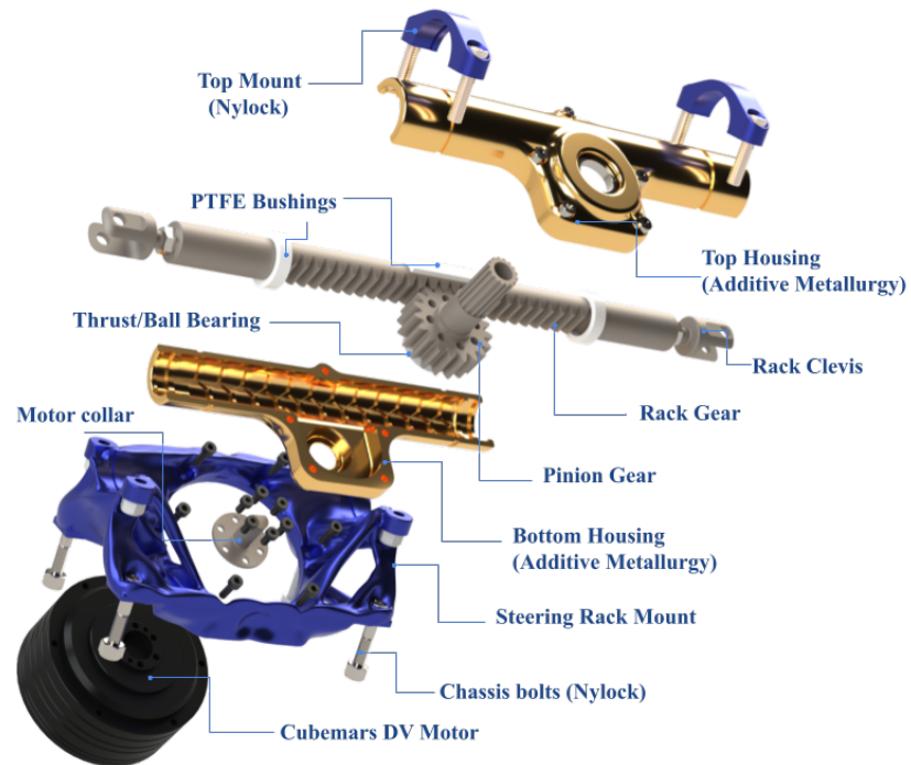
Figure 17: UT26 Steering Rack and SBW Assembly
