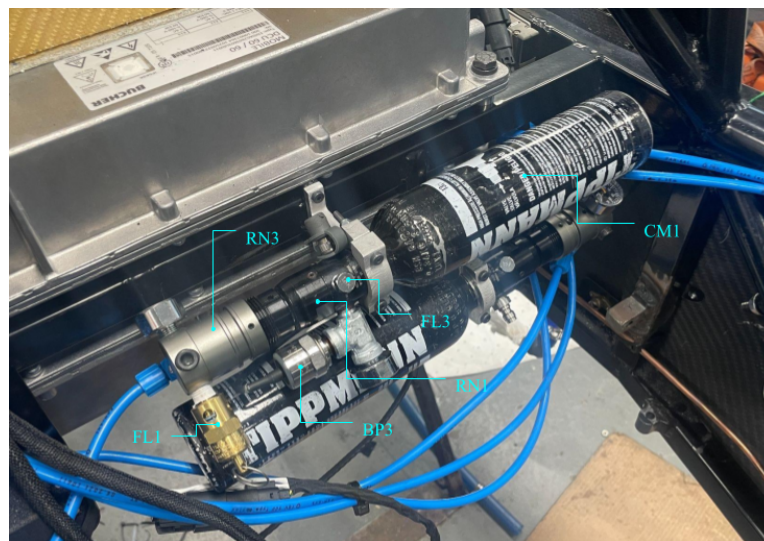
Figure 6: EBS storage tank and connected pneumatic components. Stored behind firewall.
